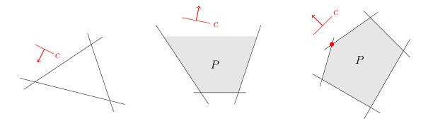
**Lemma 2.** An n-dimensional polyhedron given by m constraints has at most  $\binom{m}{n}$  vertices, i.e. finitely many.
