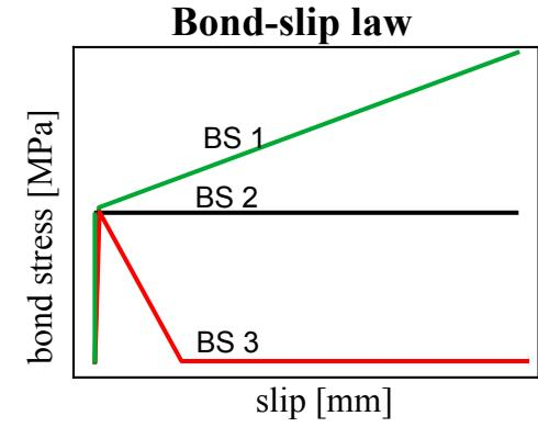
a) Associate the pull-out curve to the corresponding bond-slip law and the shear profile.
