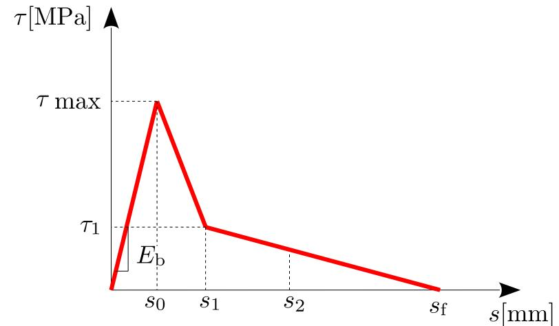
Assuming that the bond behavior is governed purely by damage and provided the characteristic points of the bond-slip law are given as
