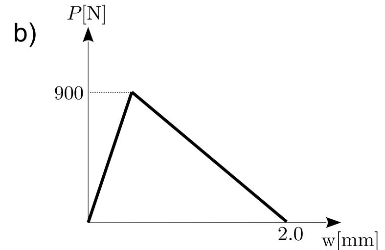
a) Determine the fracture energy  $G_f$  without considering the self-weight.
