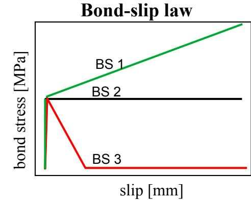
c) Assume that the behavior of the pull-out curve 1 is governed by damage, and the pull-out curve 3 is governed by plasticity, plot the unloading response at the slip  $w_1$  and  $w_2$ .
