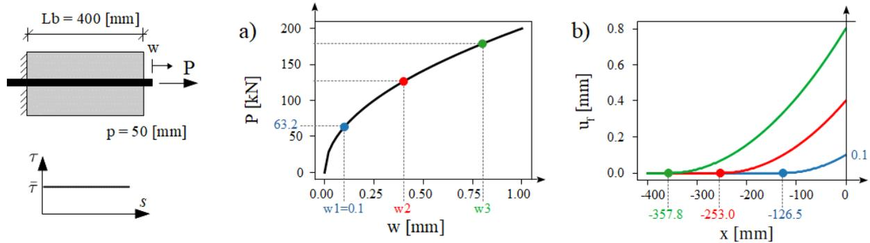
The steel rebar area and stiffness given as:  $A_f = 200[\text{mm}^2]$ ,  $E_f = 200000[\text{MPa}]$ .
