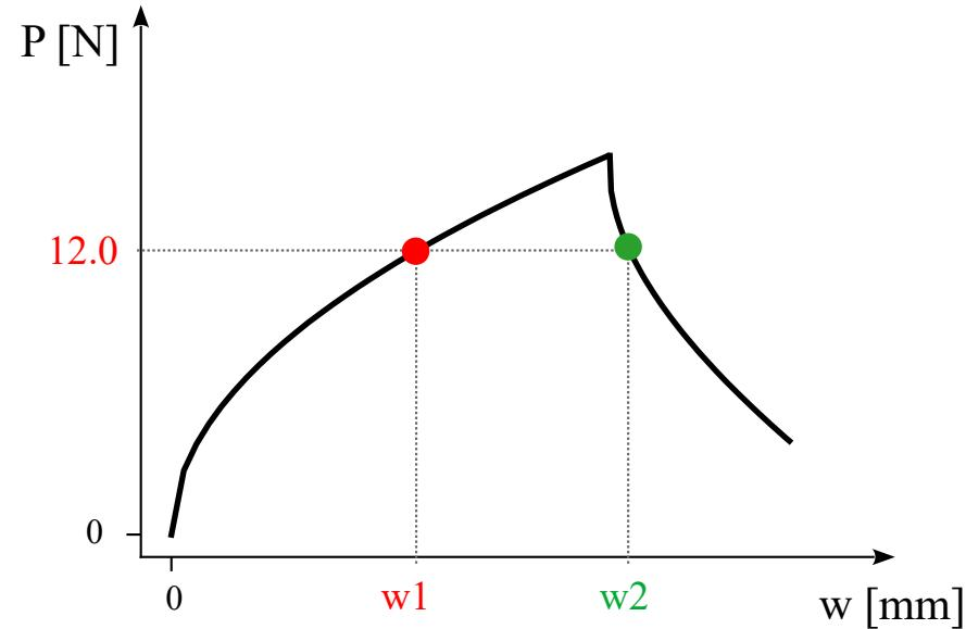
a) Calculate the debonded length ( $a$ ) at the loading stage  $w_1$ .
