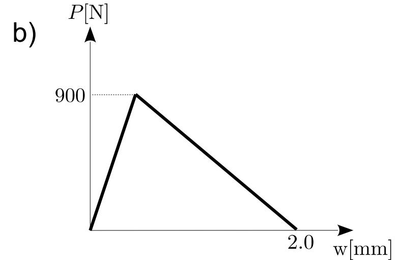
b) What would be the test response if the fracture energy was twice as large? Plot the response in terms of load deflection curve. Assume that  $P_{\max}$  does not change.
