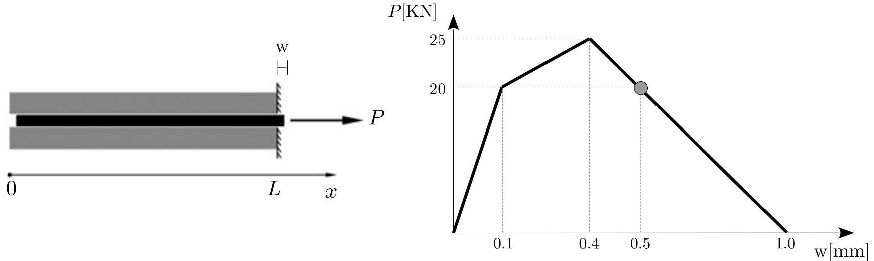
a) Evaluate and sketch the work supply, stored energy and released energy assuming that the bond-slip law is governed purely by damage.
