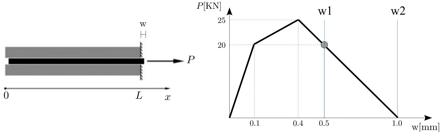
d) How to calculate the energy release rate between two points at the loading history.
